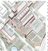
conceptual design for a new type of industrial building is being explored for the Bassett Creek Vallev Eco-Industrial Area. building The incorporates multiple levels, daylighting, solar energy harvesting and green roof technologies.
