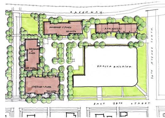
Plan view of the Shasta Building site. The design positions buildings directly adjacent to the Greenway, has interior surface and underground parking, and several different unit types.
